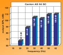
Frequency response .....40 to 113 Hz ±2.1 dB Bandwidth uniformity ..........94%
